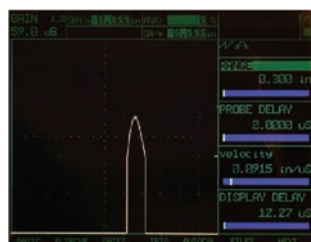
Backwall Echo from a 0.14" (3.6mm) Composite Component with ZIP
